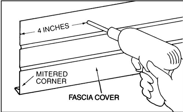
Drill nail holes in fascia cover slightly larger than nails being used. The first hole should be 4" from the end and approx. 1" from the top (Fig. 10.4). The next hole should be 22" to 24" from the end and 1" from the bottom. Continue drilling alternately every 18" to 20", leaving another 4" at the other end.
