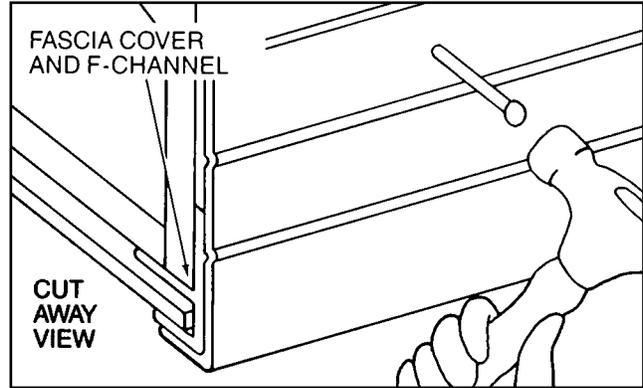
Nail through the drilled holes (Fig. 10.5). Do not drive the nails tight. Leave at least 1/32" clearance so that fascia cover "hangs" loosely. For a neater appearance, overlap fascia cover 2" to 3" and remove the bottom flange on the cover being overlapped.
