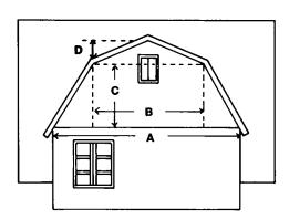
Measure the gambrel roof house as shown above to include windows and doors. Then process with the following calculations:
